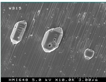
Figure 4: SEM image of three crystallites roughly 1000 to 3000 nm long. The characteristic shadowing of SEM images is clearly visible, creating the impression that the objects viewed have been lit from the side. The small particles and the stripes are 70 to 150 nm in size. (Source: Fiedeler 8 )
