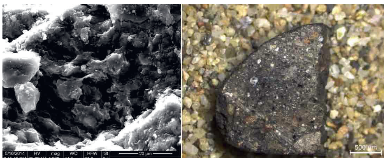
Figure 1.11. Sample MID 13/2 A: SEM image showing an unvitrified microstructure (x4000 magnification); B: image of the dark grey-black fracture of the ceramic (© C. Burke).
