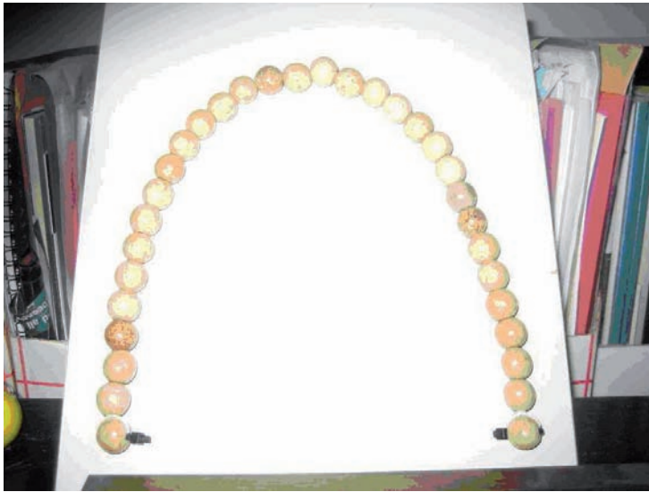
Figure 8: The ‘Inverted Chain’ experiment: a quasi-vertical arch similar to contact chains (from Duran, 1997).
