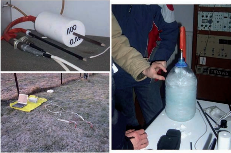
Figure 10: Tests and the test sites. The PTFE specimen with two probes under tests (top left). Two probes in snow under testing in open field conditions (bottom left). The test setup with water ice specimen (right).
