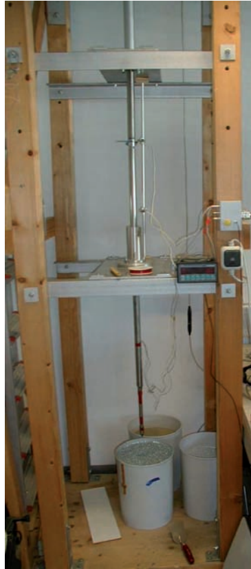
Figure 1: The penetrometry test facility used for quasi-static experiments in Martian soil analogues.
