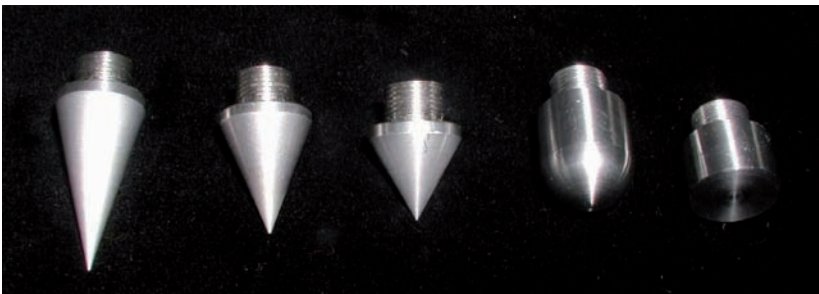
Figure 2: The standard tips used for the cone penetration test. The leftmost have a conical shape with 30^\circ , 45^\circ and 60^\circ opening angle respectively, followed by a half spherical and cylindrical shape.
