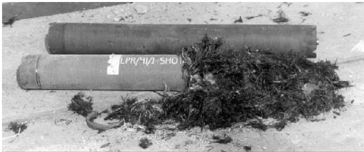
Figure 14: Aftbody on the surface with forebody buried in the ground.
