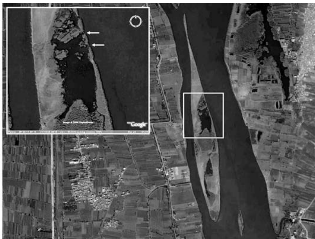
Fig. 8 Satellite image shows the location of island c. 1 km downstream of el-Lisht. The channel to the west of the island is 60–120 m wide, the island is 210 m at its widest and 1900 m long including a downstream tip that is 300 m long, but only 6–18 m wide. The close-up of the island (top left) shows a body of still water. The white arrows mark cross-bar channels, 3–5 m wide, connecting the water with the river (Images © Google Earth)
