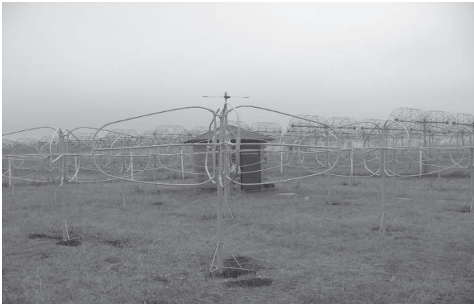
Figure 3: A 25-element GURT dual-polarised sub-array. From Konovalenko et al. [2009].
