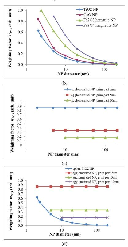
Hence, for agglomerates containing a large enough number of primary particles with a mean  $\overline{SSA_{pp}}$   $w_{PC,1}$  is also a constant  $c'_{agg}$  depending solely on the mean  $\overline{SSA_{pp}}$  of the primary particles (Figure 1c,d)
