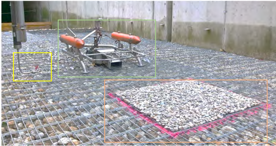
Figure 19: Flume test setup of the BfG Sampler: ADV yellow box, BfG Sampler green box and sediment sample orange box
