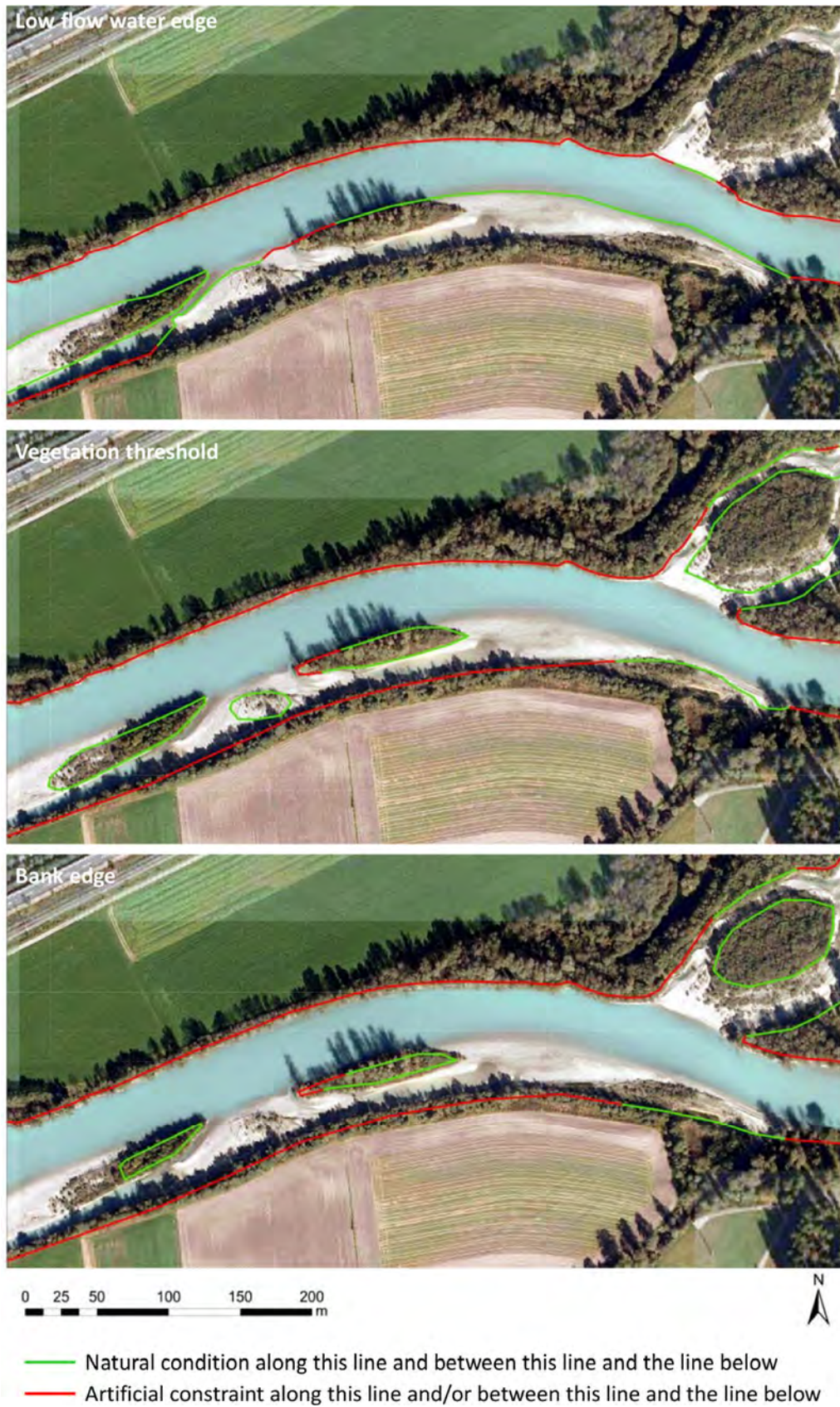
Figure 6: Artificiality along the low flow water edge, vegetation threshold and bank edge, already including buffer lengths to account for the larger-scale effect of bank protections as suggested by Klösch et al. (2019).
