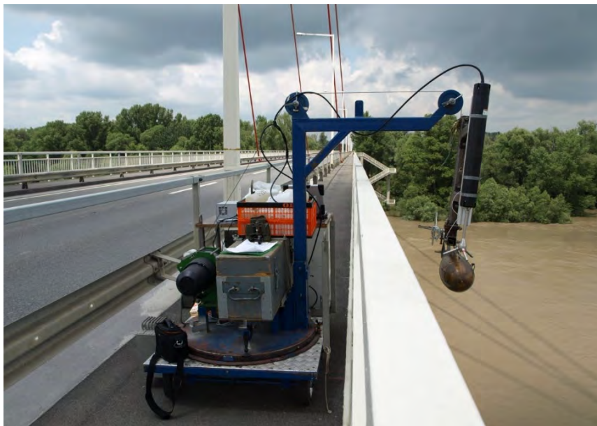
Figure 13: The trailer on the bridge with the sediment sampler and the ADV on cable (IWA/BOKU)
