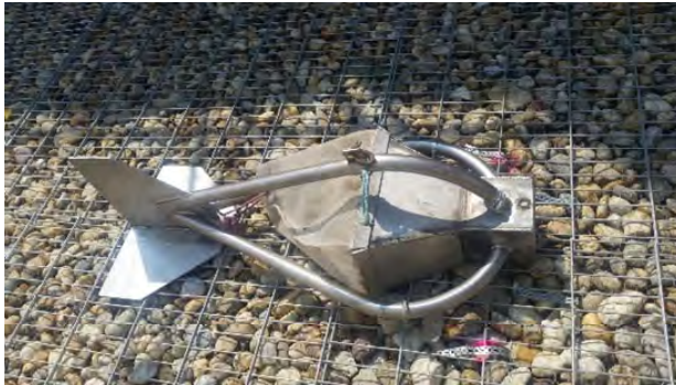
Figure 16: Large Helley-Smith sampler: mounted in the research flume (left), sketch after DVWK (Deutscher Verband für Wasservirtschaft und Kulturbau 1992) (right)
