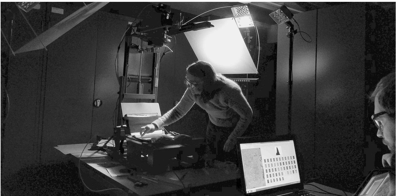
Fig. 1: The EV™ MegaVision Cultural Heritage Imaging System in use at the Staatsbibliothek zu Berlin. Dale Stewart adjusts the manuscript, while Ivan Shevchuk operates the camera. The LED panels illuminate the manuscript with one colour at a time in a series of several exposures under control of the computer (© Keith Knox)
