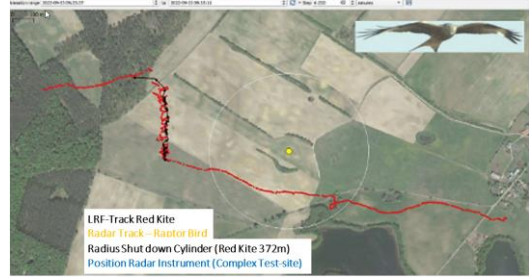
Figure 15: Example of a Radar and LRF track of a Red Kite at site 2
