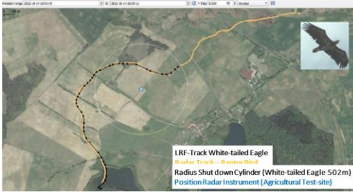
Figure 14: Example of a Radar and LRF track of a White-tailed Eagle at site 1
