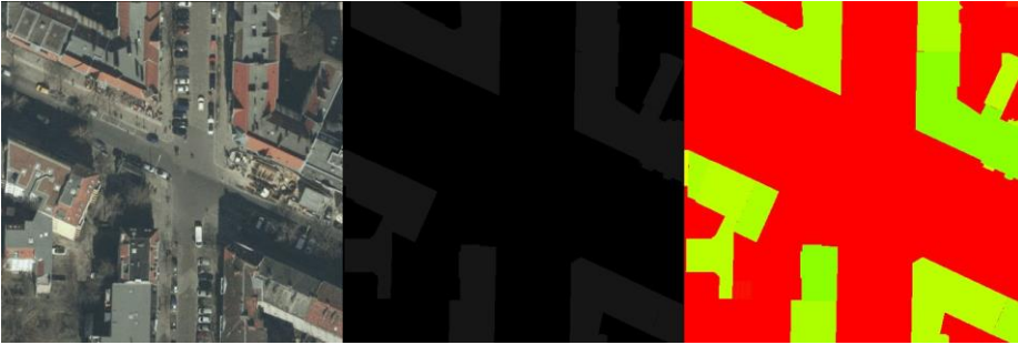
Figure 4: From left to right: Orthographic image, greyscale representation and hue representation of the height
