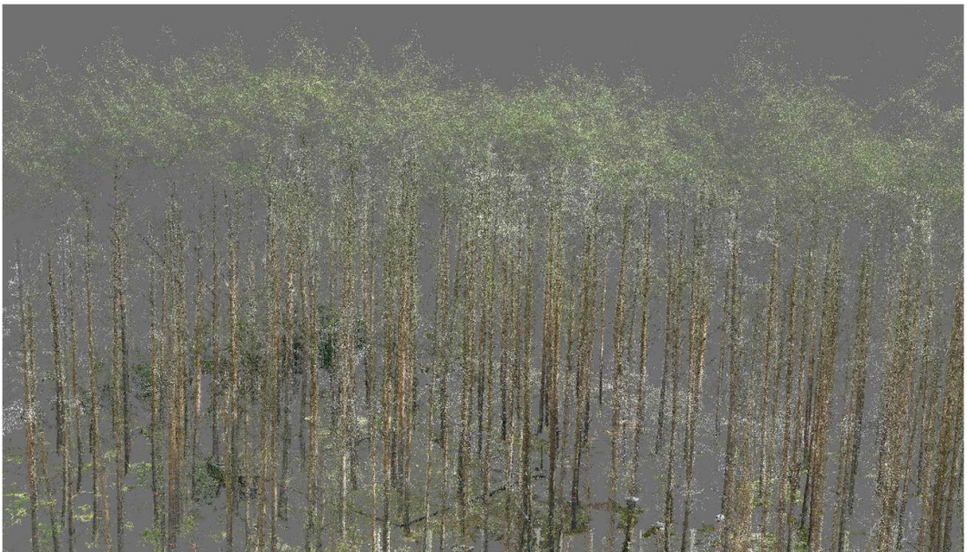
Figure 9: Oblique aerial view of the resulting merged point cloud. White points in the upper canopy are due to noise propagated from sky in the terrestrial imagery
