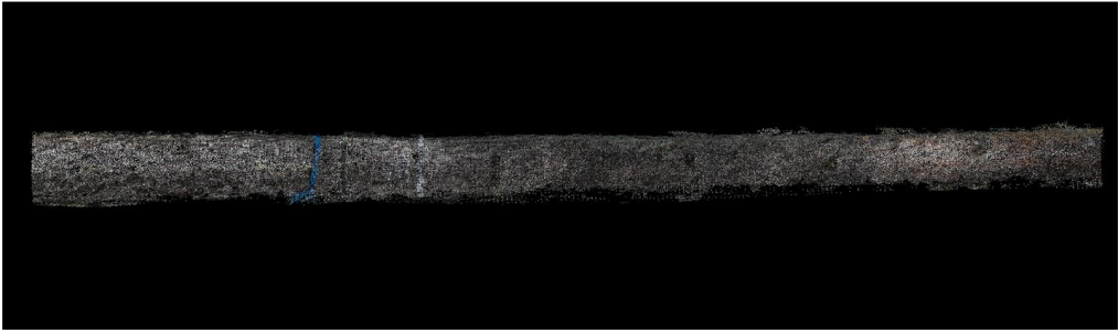
Figure 11: Tree stem (RGB) segmented at 4 m with the manual removal of extraneous points
