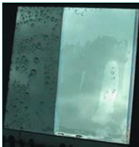
Figure 5: Hydrophilic coating (right) with TiO 2 on float glass ( www.wopag.uni-bayreuth.de )
