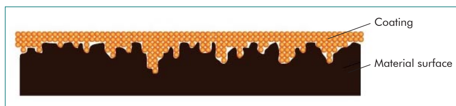
Figure 4: Diagram of an “Easy-to-Clean” surface ( www.nanoprotect.de , 30.4.10)
