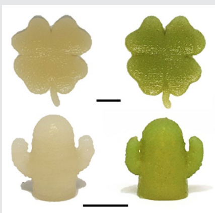
(b) Microalgal in a hydrogel scaffold, ELMs in the shape of cacti and clovers 14 days after incubation under autotrophic conditions.
