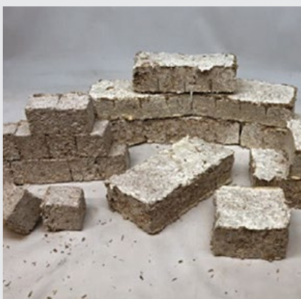
(d) Sterile Ganoderma sp. is combined with raw non-sterile feedstock and grown in a mould before the form-stable moulded biocomposite is post-processed 10 .
