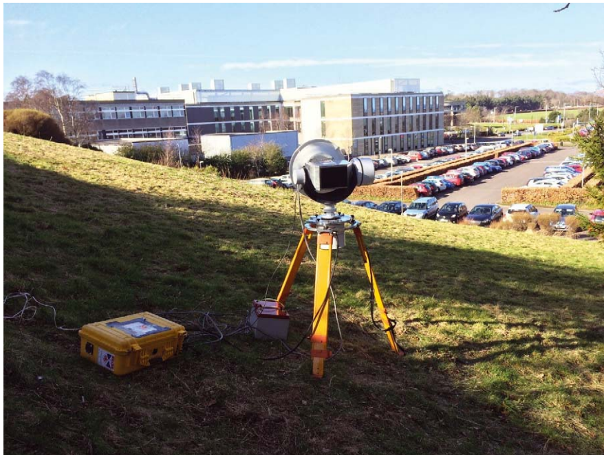
Figure 1: The AVTIS millimetre wave radar. Photograph: William D. Harcourt, 2019.
