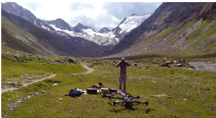
Figure 1: Unmanned Aerial Vehicle laser scanning in Rotmoos Valley (Ötztal, Austria). Photograph: Rutzinger, M. 2018.
