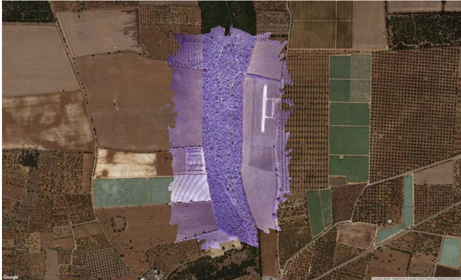
Figure 1: Example of orthomosaic georeferenced using GCPs from the Google Maps source (Image © 2018 DigitalGlobe, European Space Imaging).
