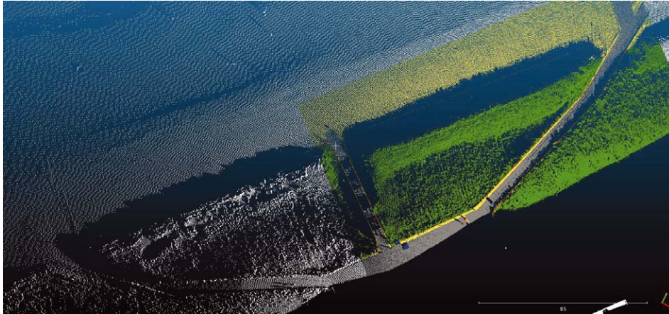
Figure 1: Point cloud of the beach at Kijkduin on 01.01.2017 with surface classification for a selected area. Yellow points represent dry sand, green points represent the dune area, pavement is coloured in grey and people and buildings are shown in red and blue respectively.
