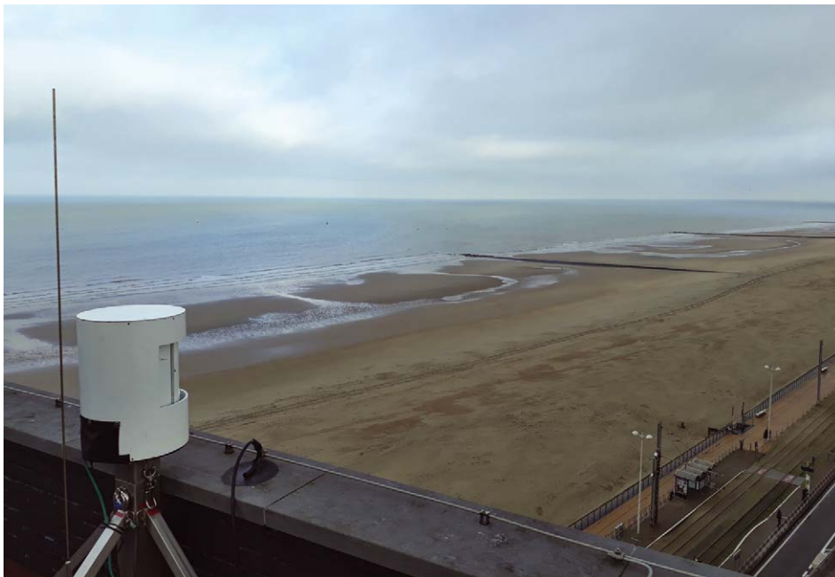
Figure 2: The Riegl VZ-2000 laser scanner on top of a building in Oostende, Belgium. Photograph: Roderik Lindenberg.
