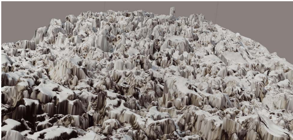
Figure 2: Example of SfM 3D model of a section of Wahlenbergbreen, Svalbard, made from sUAS-data from field work during summer 2018, processed with Agisoft Photoscan software. Images for the model recorded with DJI Mavic Air. © Endre Før Gjermundsen
