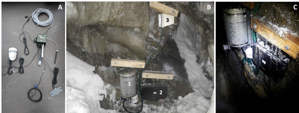
Figure 19: (A) Assembling tests of miniature weather station (Libelium Smart Agriculture Xtreme 1.0) connected to all five sensors; (B) Weather station installed at MS Randkluft Dark inside a robust aluminum housing (1), connected to external 4V battery (2) and external antenna (3); (C) Weather station covered with thin layer of ice ('verglas') after a one-year test run inside the randkluft (MS Randkluft Dark).
