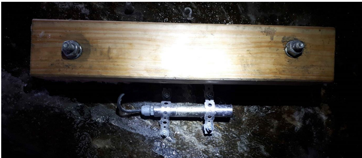
Figure 4: Miniature temperature logger (Geoprecision M-Log5W-Rock) installed 7 m below the glacier surface ('Randkluft Deep'). The wooden beam protects the logger from falling ice and rocks.
