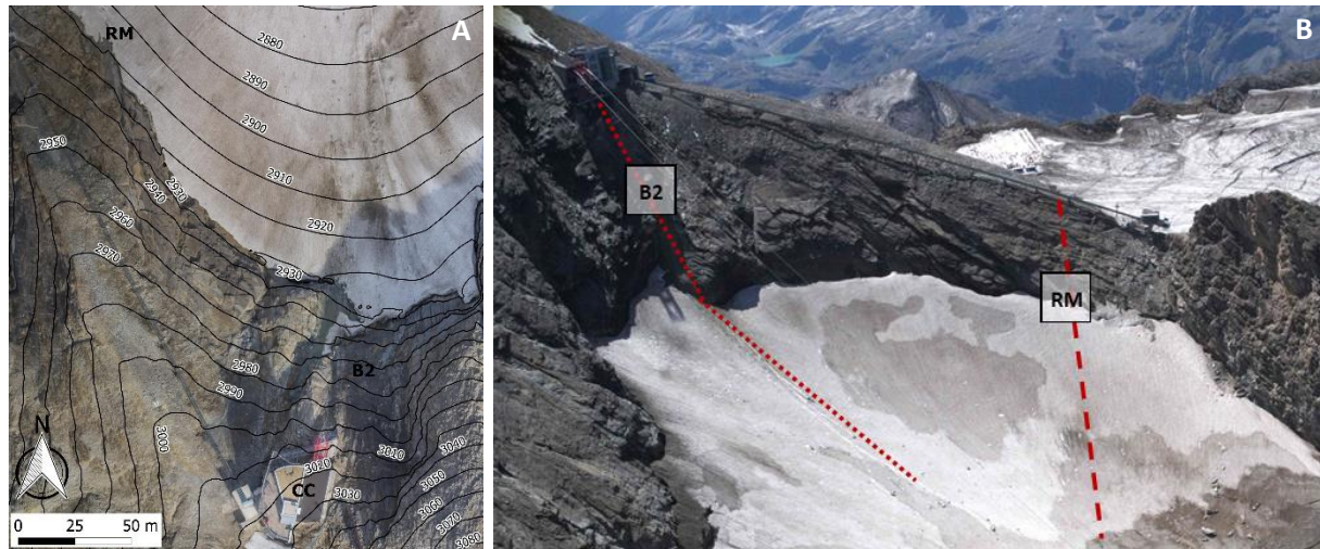
Figure 2: (A) Orthophoto of study site; (B) Oblique view of the investigated glacier-headwall system. Dotted line: 2D profile line used for Figure 5A; Dashed line: 2D profile line used for Figure 5B (Photo: R. Delleske, 24.08.2017). Abbreviations: (RM) Randkluft Monitoring; (B2) Borehole (30 m); (CC) Cable car top station.
