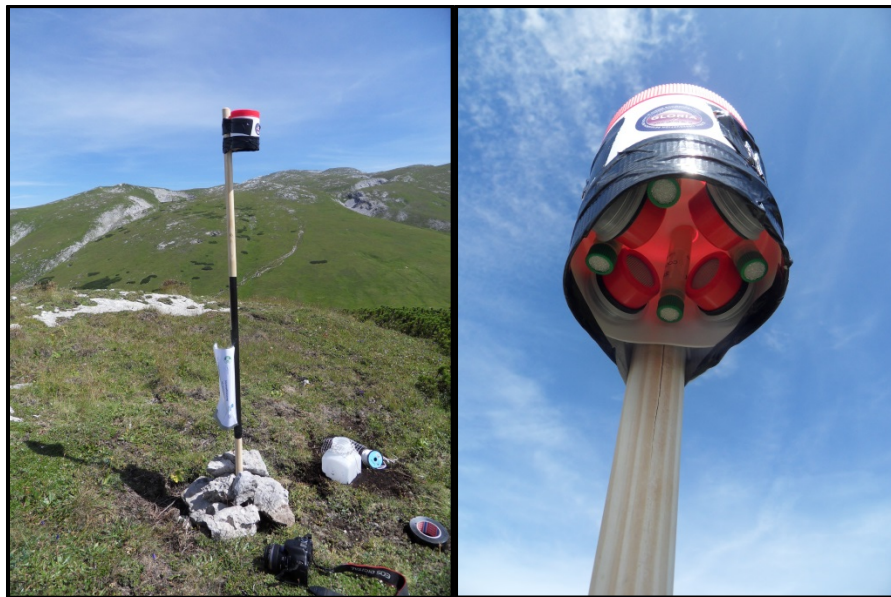
Figure 9. Nitrogen deposition sampler unit ( \text{NH}_3 and \text{NO}_2 ) on Mt. Hochschwab
