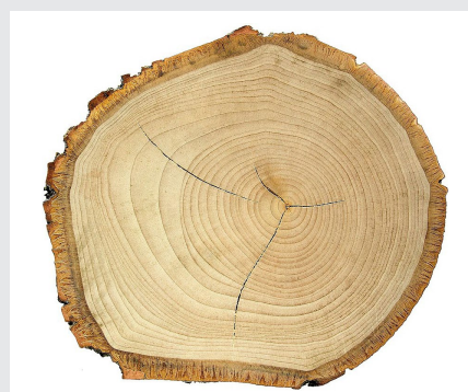
(c) Cross-sectional view of a Silver Linden tree, exhibiting a diameter of 190 mm, employing both compression and tension wood regulating and optimizing structural strength 30 .
